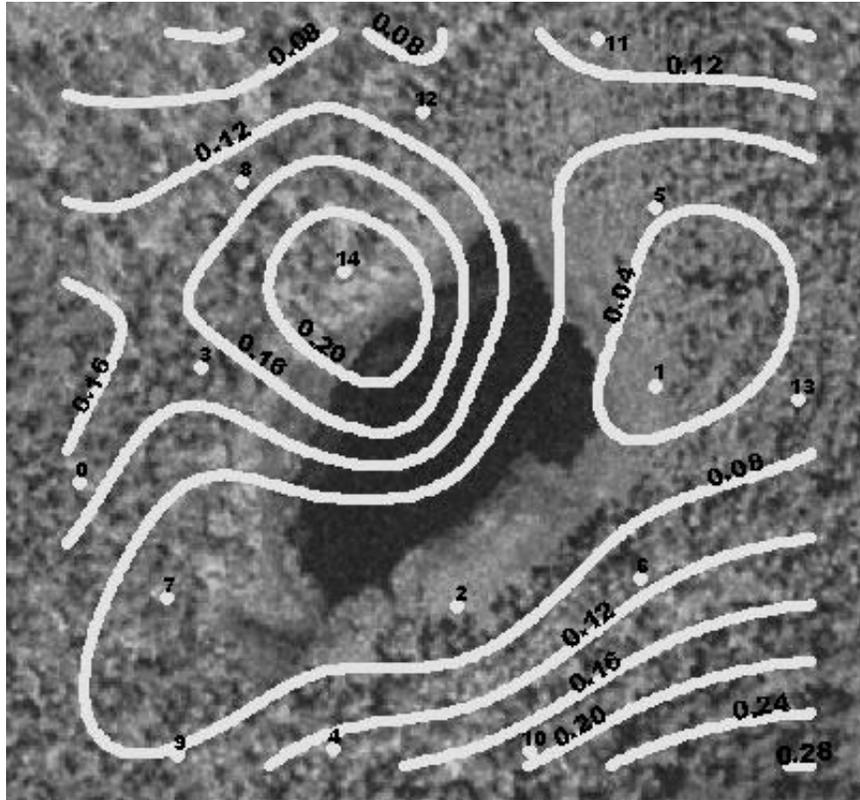
**Figure 8.** Specific conductance contours (mS/cm) on 11-17-01 at Molly bog.
