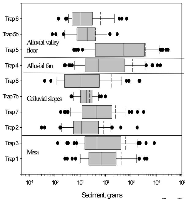
Figure 5. Storm event generated sediment measured in the sediment traps. Locations of traps shown in figure 4b.
