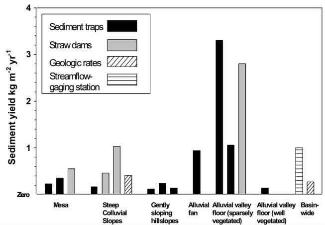
Figure 6. Sediment yield measured using sediment traps and straw dams on the geomorphic elements defined for Arroyo Chavez Basin, basinwide erosion using suspended-sediment loads measured at the streamflow-gaging station, and geologic rates of erosion using  $^{10}\text{Be}$  (Clapp et al., 2001).
