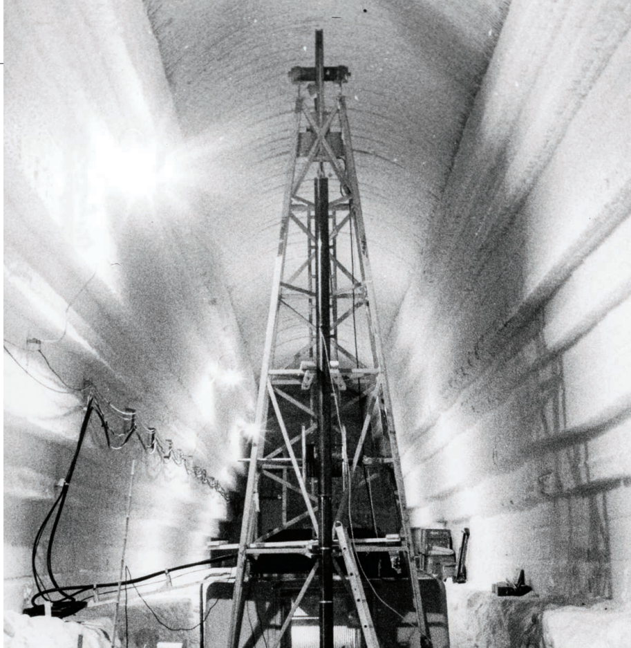
A 9-meter rig in Camp Century's secret ice tunnel drilled a core that is still yielding discoveries.
