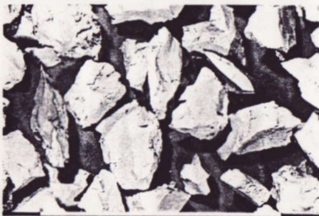
Fig. 2. Final result of the separation procedure, showing pure quartz. The scale bar is 1 mm.
