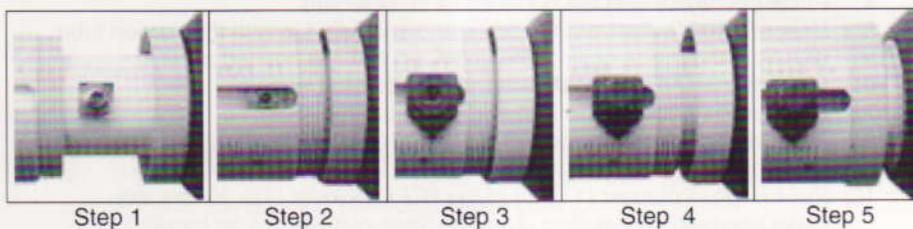
9. Erect the device and push the glass plunger (17) into the PTFE cylinder (18) until it stops.
