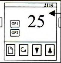
**Measured Chamber Temperature**
