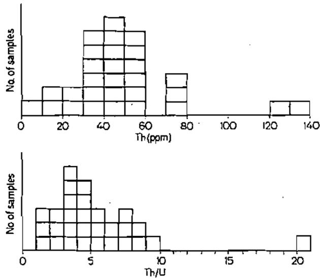
Fig. 90-K-2. Histograms of thorium concentrations and Th/U ratios in a world-wide sampling of bauxites. (From ADAMS and RICHARDSON, 1960)
