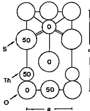
Fig. 90-A-1. The atomic arrangement in ThOS (PbFCl-structure) projected along one of the *a*-axes (FERRO, SR 1955, 289)
