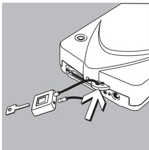
**Antitheft Locking Device on Balances with a Weighing Capacity up to 10 kg**
