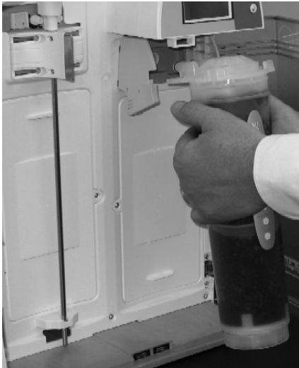
Quantum Cartridge being pulled out from the pack adapter.
