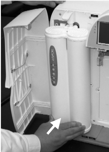
Q-Gard Pack pushed in at the bottom.
