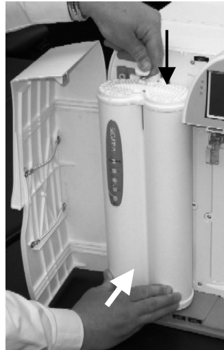
Pak Locking Handle being pushed down while holding the bottom of the Q-Gard Pack.
