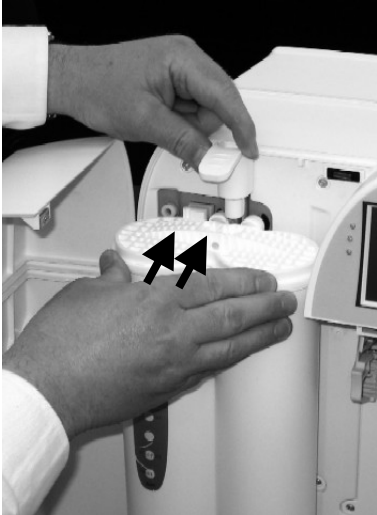
Pak Locking Handle being pushed down while holding the bottom of the Q-Gard Pack.
