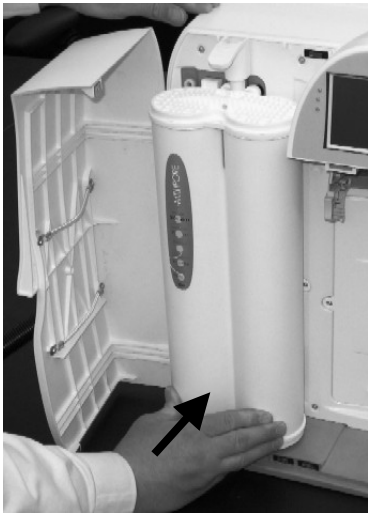
Q-Gard Pack pushed in at the bottom.
