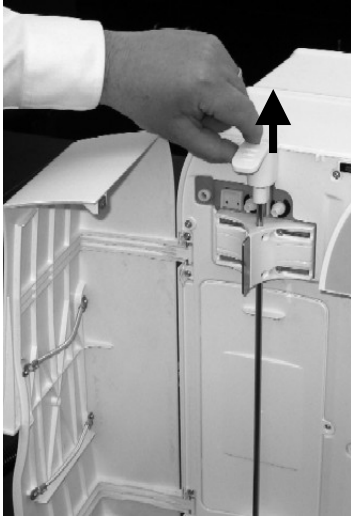
Pak Locking Handle lifted up.
