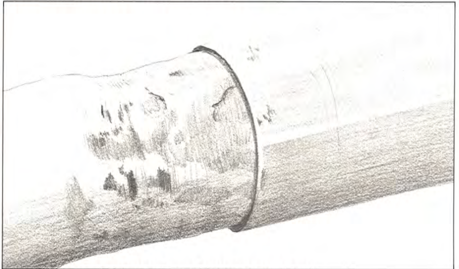
Metal burrs on a bent guard could cause an accident
