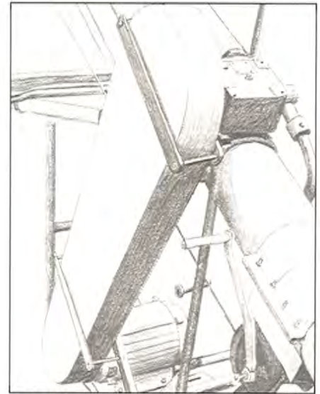
Properly guarded sheaves and belt
