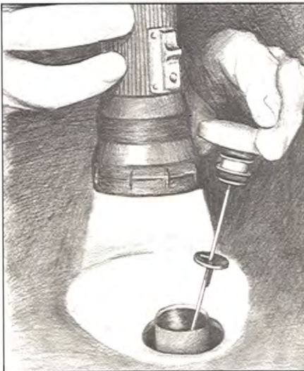
Shine flashlight into reservoirs
