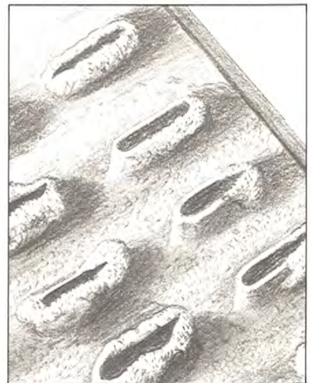
Severe radiator corrosion
