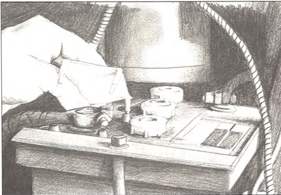
Terminal posts on batteries should be protected
