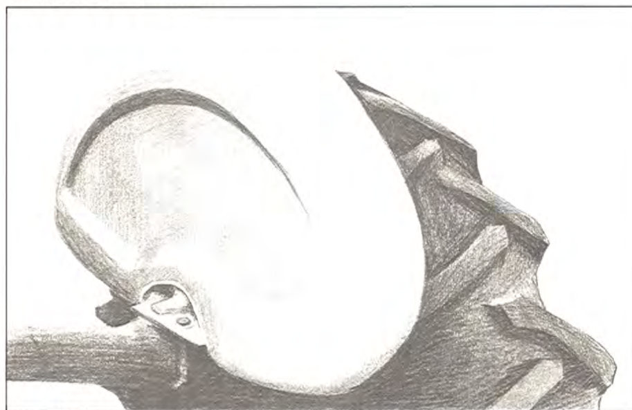
Fenders protect the driver from flying objects
