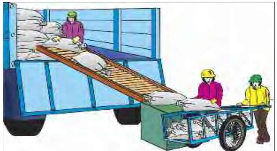
Figure 11e. Use roller-conveyers to move heavy objects over short distances.
