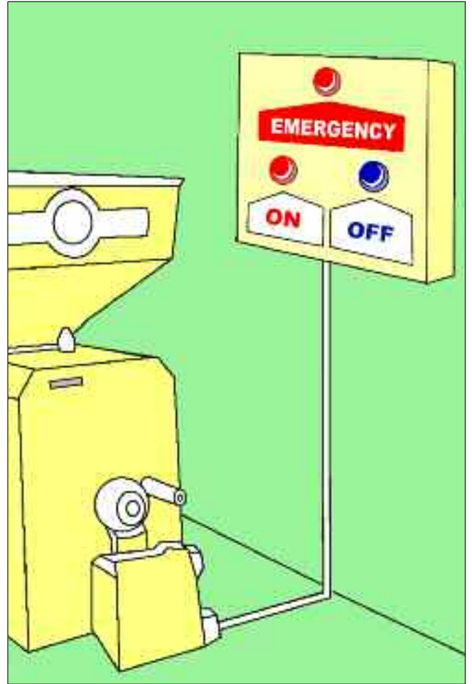
Figure 35b. Electrical cables connected to the machine are well protected and clearly labelled.
