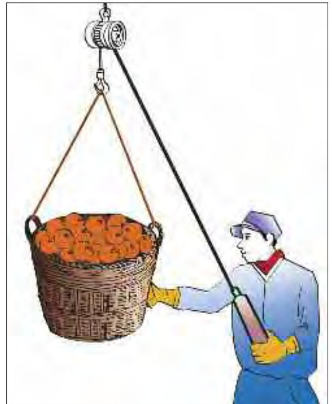
Figure 11b. An electric chain hoist with a control switch, used for efficient lifting of heavy loads.
