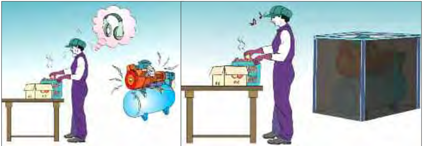
Figure 55a. Workers working near a noisy machine should be protected by placing it in a soundproof enclosure.
