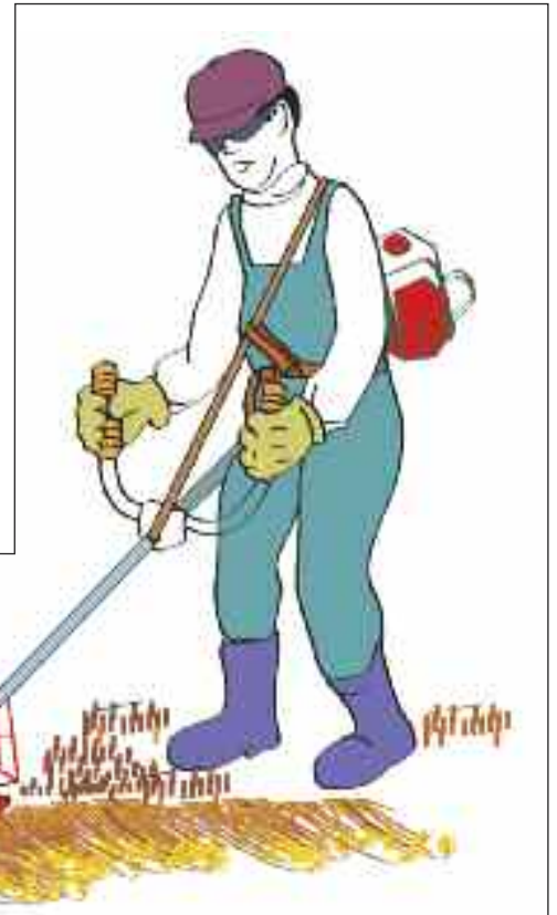
Figure 24b. Use a hand-reaping machine to reduce the workload on your arm and hand muscles. Attach sturdy handgrips to the tool to secure a safe grip.
