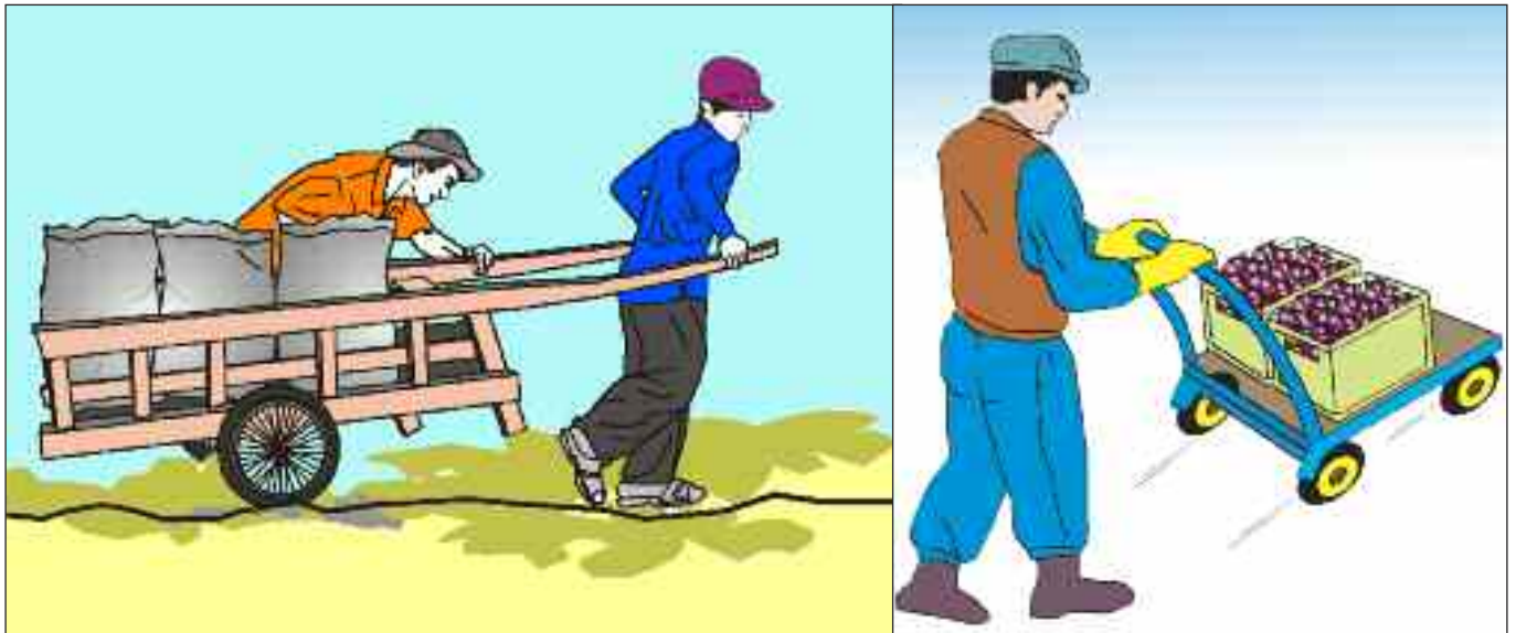
Figure 5a. On rough roads, it is easier to push or pull hand-trucks with large wheels (left) than those with small wheels (right).
