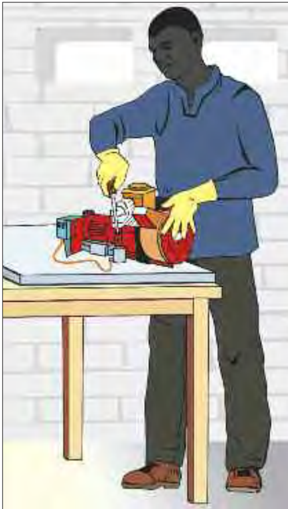
Figure 27a. Adjust work tables to allow for the right work height according to the type of work being done.
