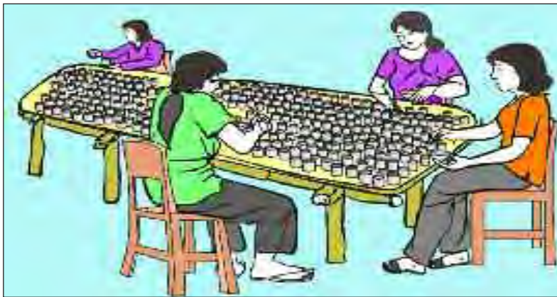
Figure 23b. Change work that is usually done at ground level, such as raising young trees or sorting farm products, so that it can be done in a seated position, with the working surface corresponding to elbow level. Use comfortable chairs with backrests.
