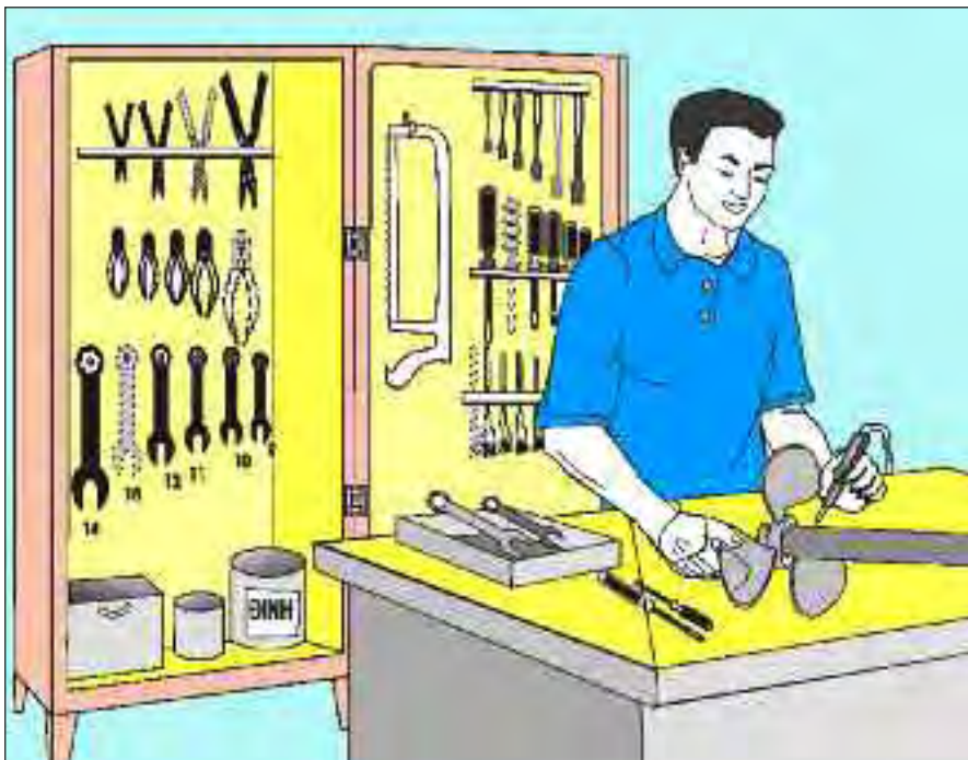
Figure 15a. Provide tool storage cabinets near the work area, within easy reach.
