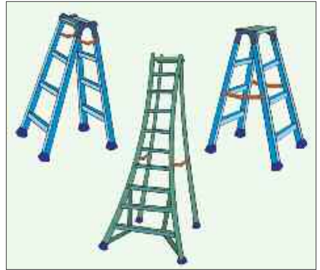
Figure 28b. Stepladders of different shapes are available. Use ladders with arrangements for avoiding sudden collapse.
