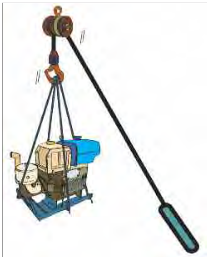
Figure 38a. Fix the load safely when it is being lifted by a hoist or a crane.
