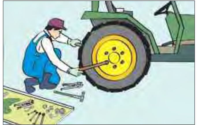
Figure 34b. Pay special attention to dangerous parts of the machine. Ensure that the machine is switched off during maintenance.
