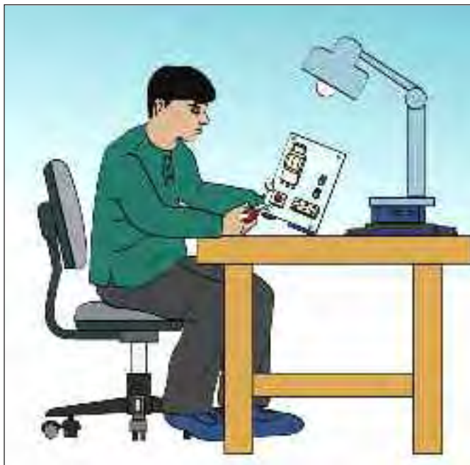
Figure 50c. Provide a task light for precision work. You can check the appropriate position for the light by considering the type of work done.
