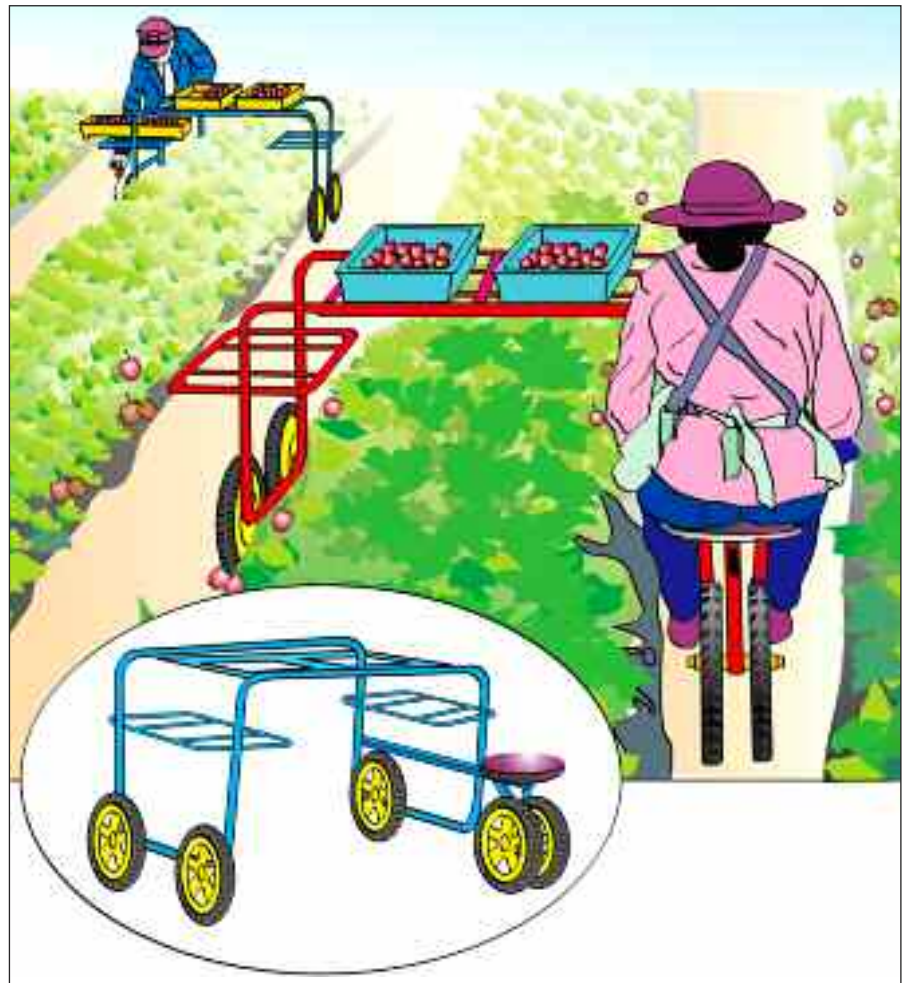
Figure 5c. A comfortable strawberry-picking vehicle with a wheeled work-seat.
