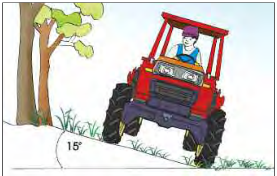
Figure 47c. Avoid operating an agricultural vehicle along a slope exceeding 15 degrees.
