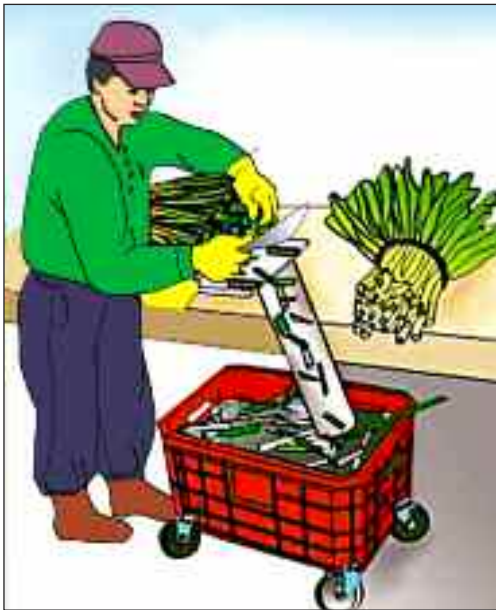
Figure 14a. Provide waste containers that are conveniently placed and easy to empty.
