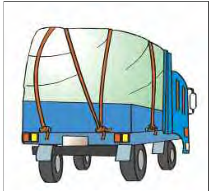
Figure 46b. Covers for materials or products carried are useful for preventing damage and falling.
