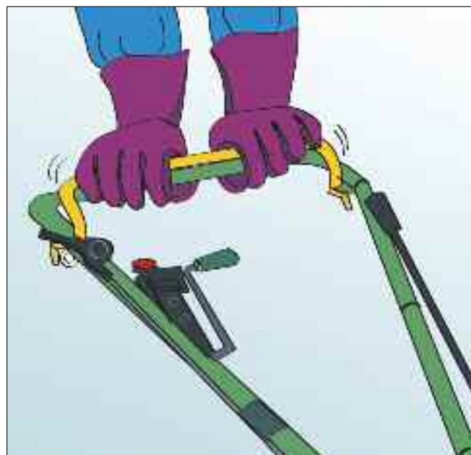
Figure 37b. Select a machine that stops automatically when the control is released.
