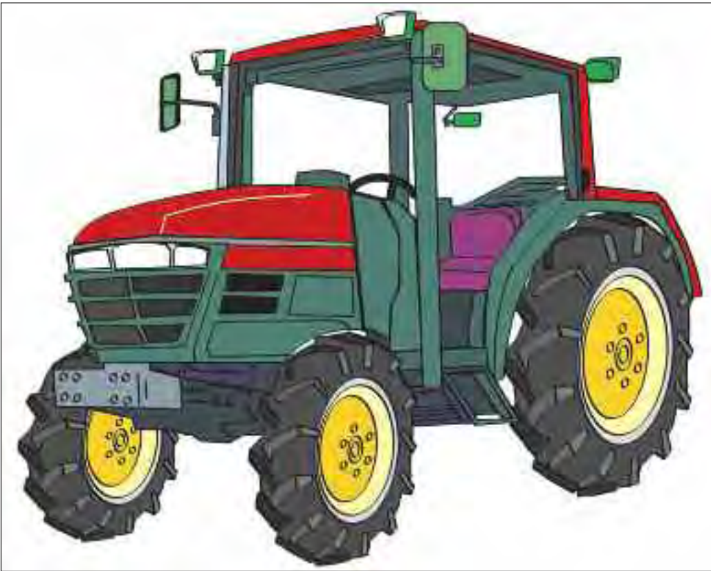
Figure 45b. Easy access to the driving seat is also important, as are measures to reduce noise and vibration, to increase seat comfort and to avoid mistakes in operation.
