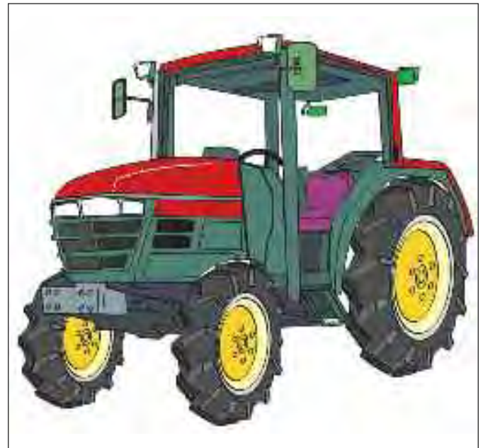
Figure 48b. Mirrors can increase the front and rear views for the driver.
