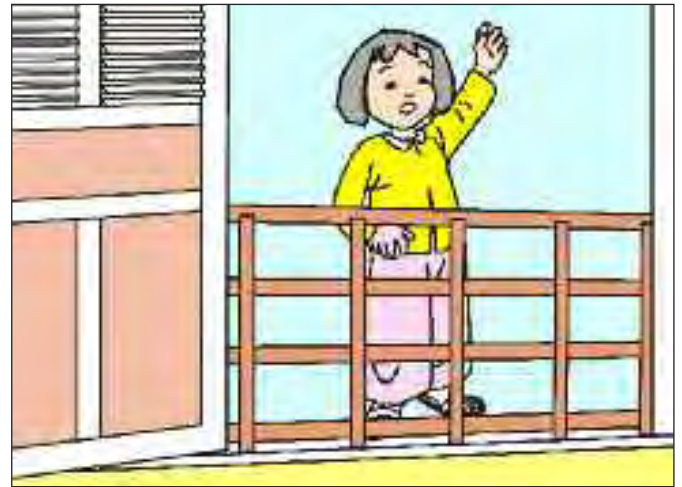
Figure 76b. Safety frame to keep children inside the house. The frame is removable for ease of access.
