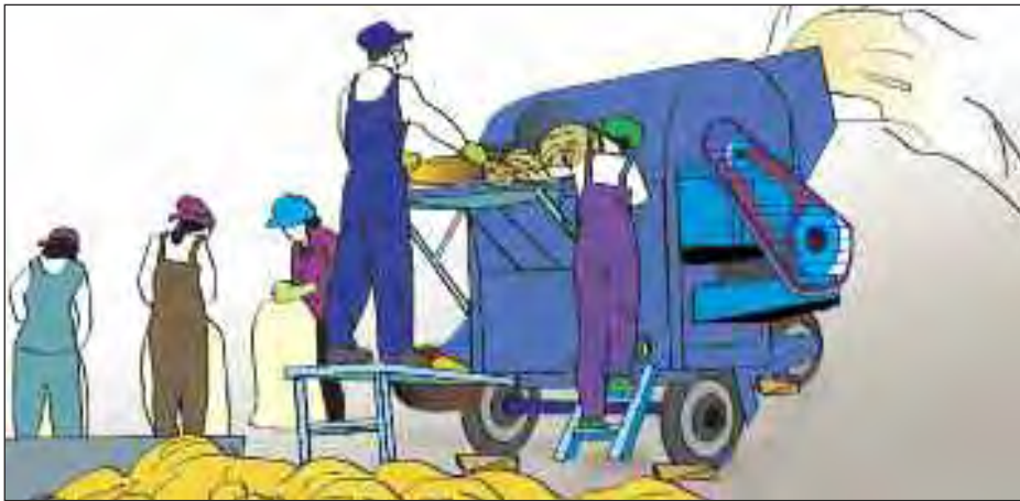
Figure 32a. Use wedges to fix machines with wheels, or use machines with caterpillar tracks.
