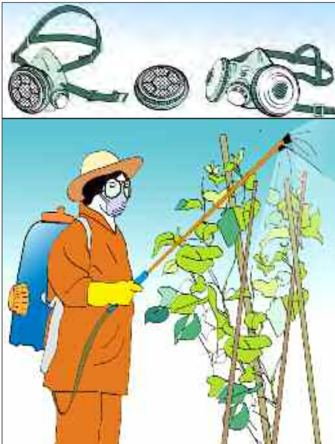
Figure 65c. Mask, with filter containing granules of activated carbon, for use when spraying with pesticides.
