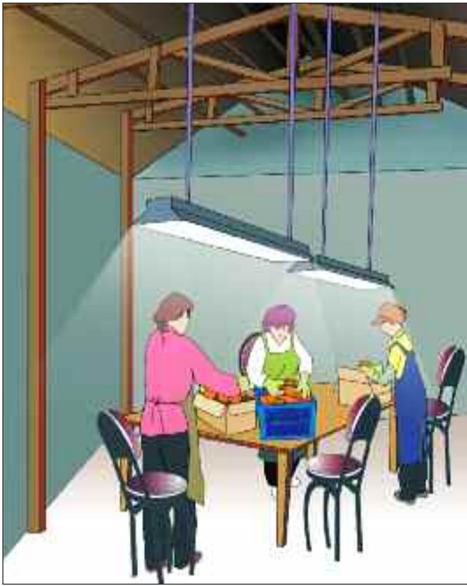
Figure 50a. Relocate lights to obtain sufficient lighting for precision or inspection work.
