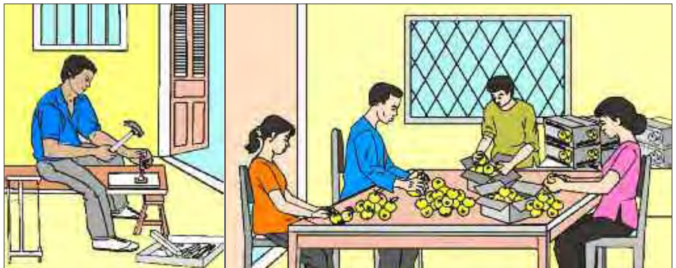
Figure 49c. Position workstations near to doors or windows to take advantage of daylight.
