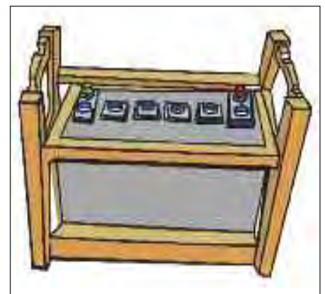
Figure 9d. A battery contains dangerous chemicals. Put it in a container with safe, firm handles.
