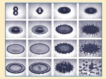
on a hot metal surface. Whether each droplet spreads, splashes or rebounds depends on its impact energy as well as on the temperature and roughness of the surface.
