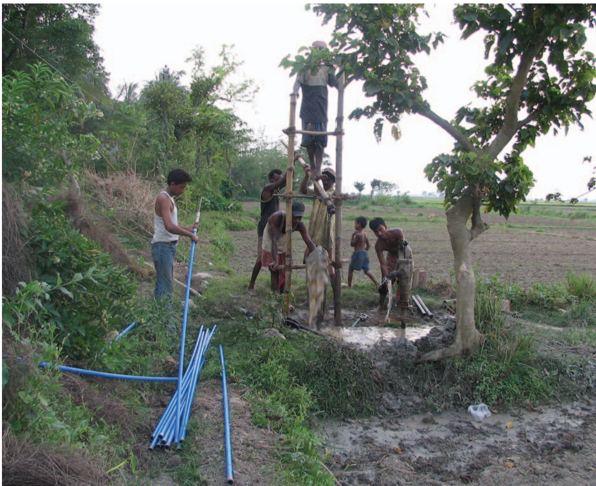
FIGURE 4 Needle sampler and narrow-gauge casing being used in West Bengal to sample groundwater down to depths reaching several tens of metres. These needle samplers (van Geen et al. 2004) obviate the need for a full-size well to be drilled; they allow sampling of both water and particulates under anoxic conditions at different depths, and thus readily enable on-site testing for groundwater arsenic at potential well sites. These samplers will be of particular use in implementing well switching as a short-term remediation strategy.
