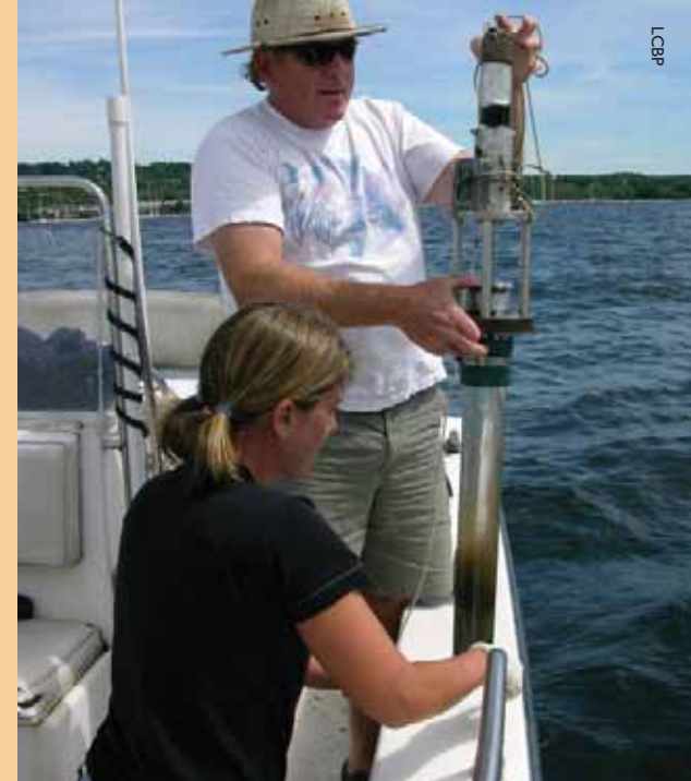
A CORE OF SEDIMENT from the Lake bottom is taken to test for mercury and other toxins.
