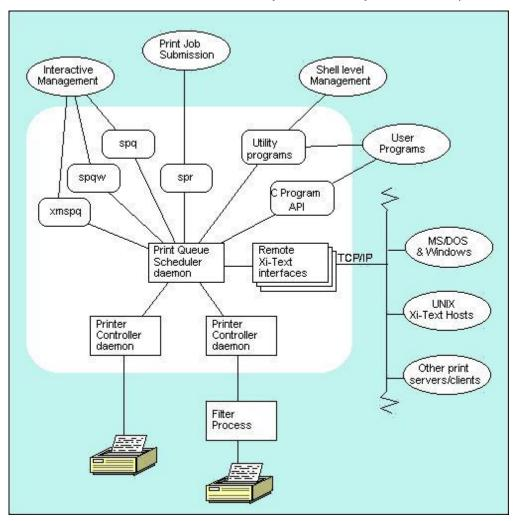
At the heart of **Xi-Text** is the print queue scheduler daemon <u>spshed</u>, which manages the print jobs. There is one instance of <u>spshed</u> running on a stand alone system, or two if co-operating with other **Xi-Text** hosts. Co-operating **Xi-Text** hosts require a network providing TCP/IP services.
