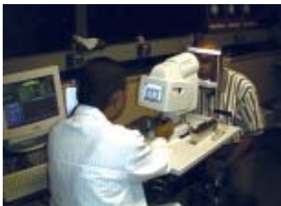
Dr. Ansari and an ophthalmologist perform a clinical test using a Dynamic Light Scattering Device that determines molecular interactions that occur in the human lens.
