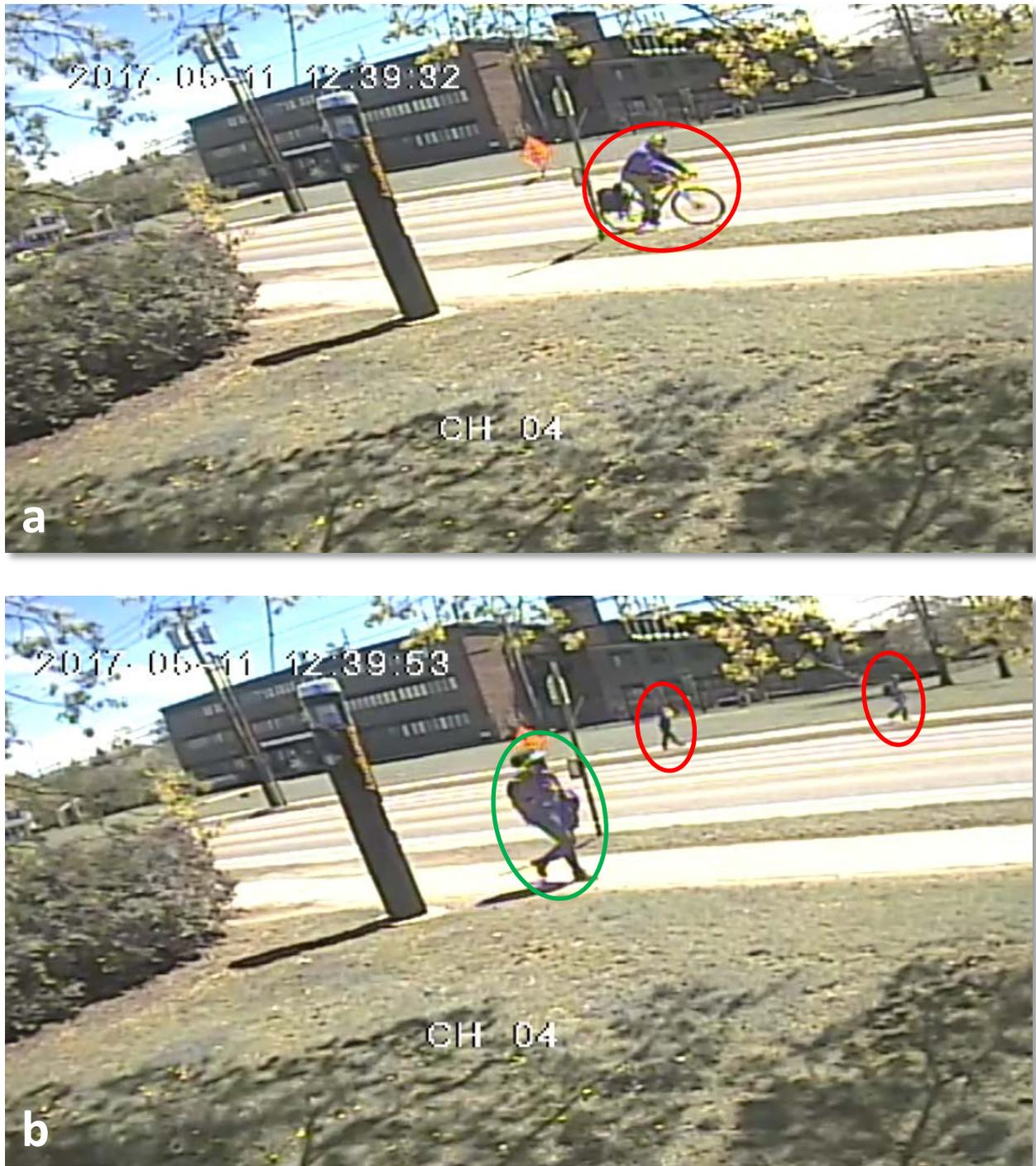
Figure 36. a) Bicyclist passes the infrared counter on a bike lane in the traveled way. b) Pedestrians on the opposing sidewalk are missed by the placement of the EcoCounter
