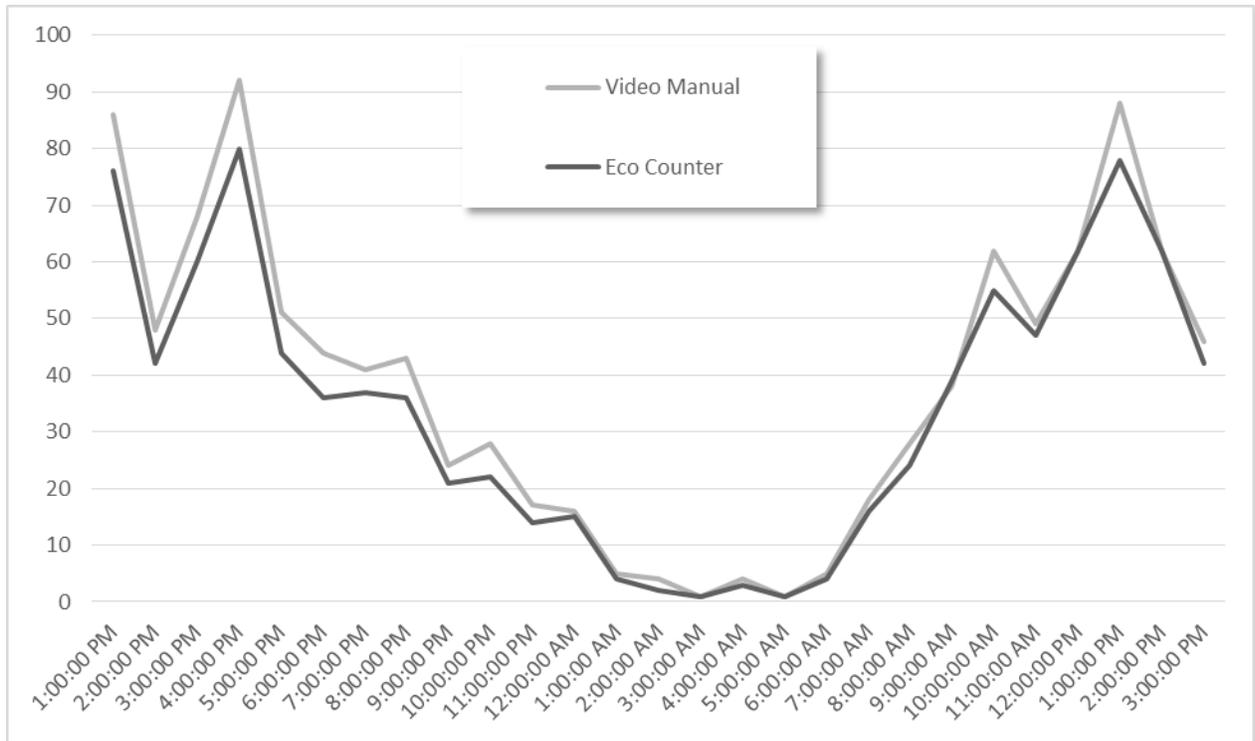
Figure 34. Video-based manual and EcoCounter count comparison.
