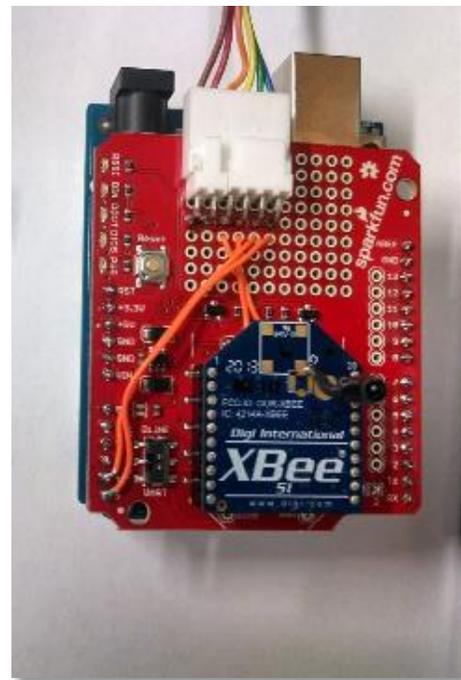
*Figure 3.6: Accelerometer (red) and Arduino Pro Mini (blue)*      *Figure 3.7: Arduino Uno (red) and Xbee (blue)*
