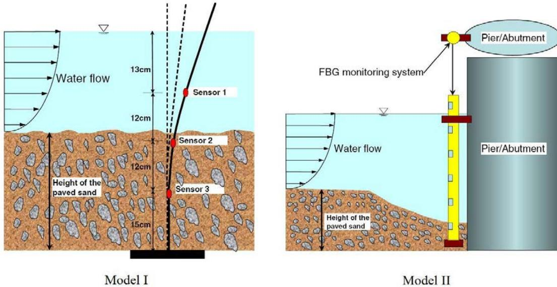
Figure 3.2: Fiber Optic Scour Sensor (Cai et al. 2014)
