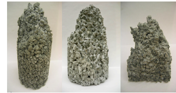
Porous concrete samples after compression testing: Lab Mix #1 (left), Lab Mix #2 (middle), Field Mix (right)
