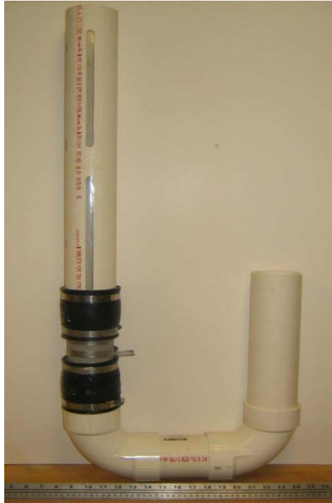
2 3 4 5 6 7 8 9 10 11 12 FIGURE 1: Falling Head Permeameter.
