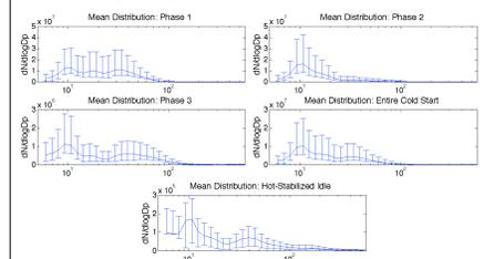
**Figure 5:** Mean particle number distributions, where the solid line is the average and the error bars represent the overall range for all 5 sampling runs.
