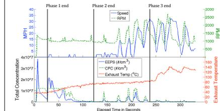
**Figure 3:** Vehicle parameters and particle number concentrations (#/cc) from EEPS and CPC, displaying different observed phases of cold start.
