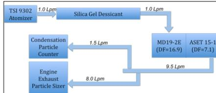
**Figure 1:** Schematic of and the corresponding flowrates of the laboratory setup for particle instrument validation.
