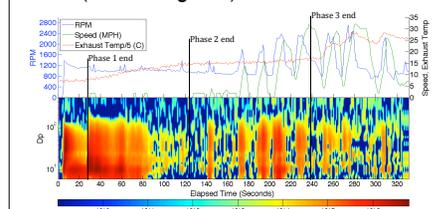
**Figure 4:** Time series EEPS particle number distribution (colorbar scale is dN/dlogDp). Figure is corrected for instrument noise.
