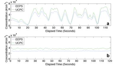
**Figure 2:** Transient (a) and constant (b) concentration tests results
