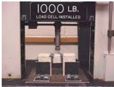
Shear test on foam sealant using Instron testing machine.
