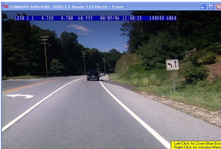
Example location with left turn lane on a horizontal curve
