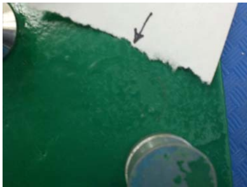
Figure 2. Paint B7-97 on galvanized steel after pull off at 680 psi.
