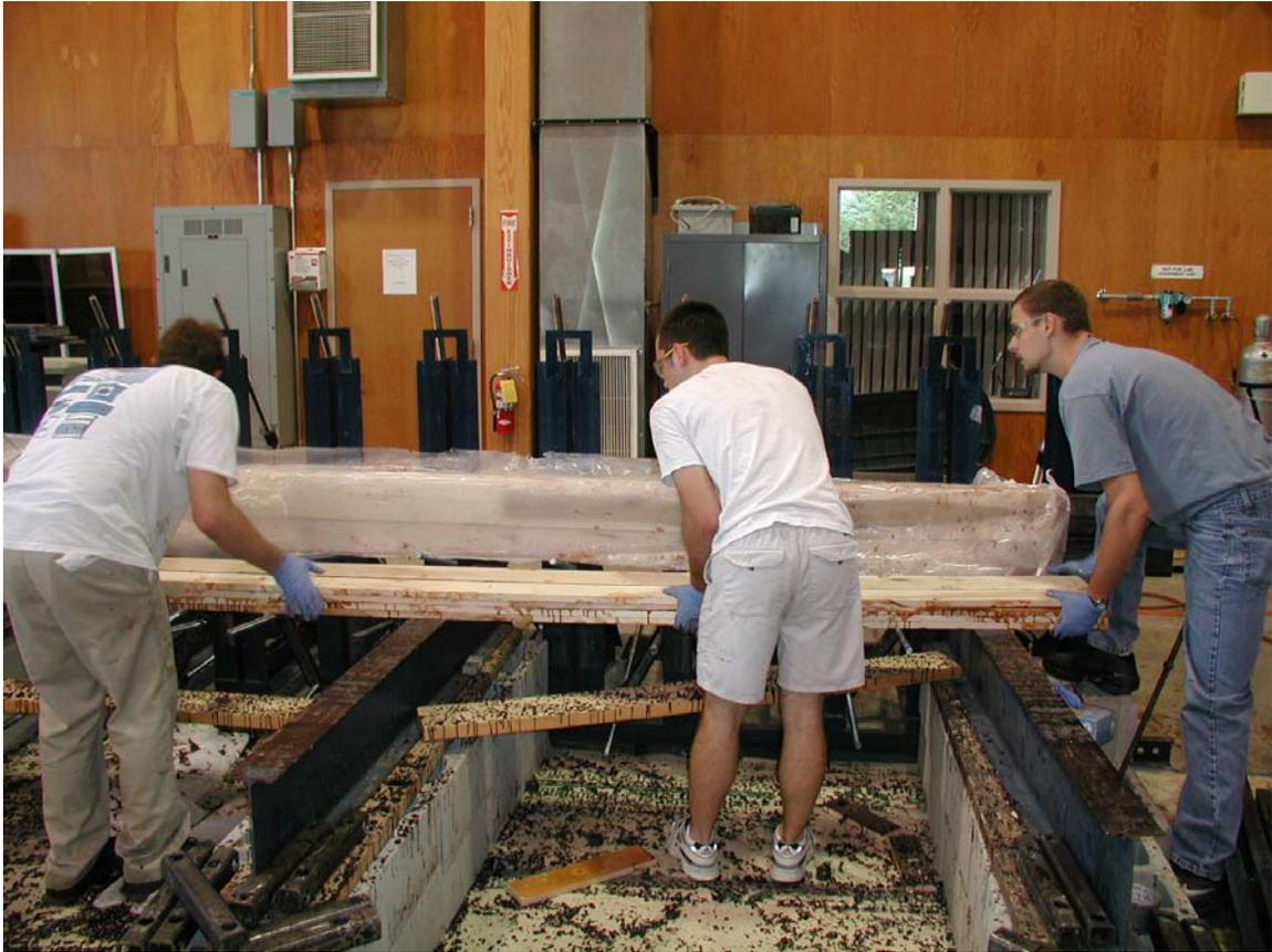
Figure 1: Guardrail Layup in Progress
