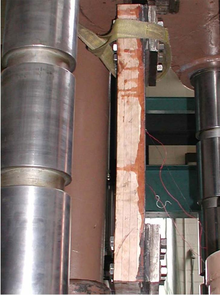
Figure 2: Rail Tension Splice Test
