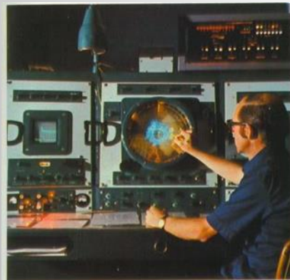
Milt and Joan Marin Weather radar helps meteorologists detect areas where rain is falling. Radio waves sent out by a radar system are reflected by raindrops, and the rainy areas appear on a screen, above.
