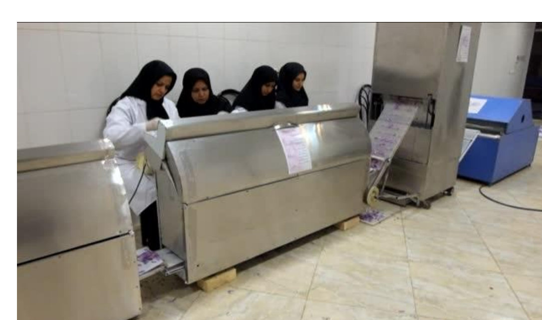
A saffron separating machine in a factory. The process has not been fully mechanized, but throughput is increased.
