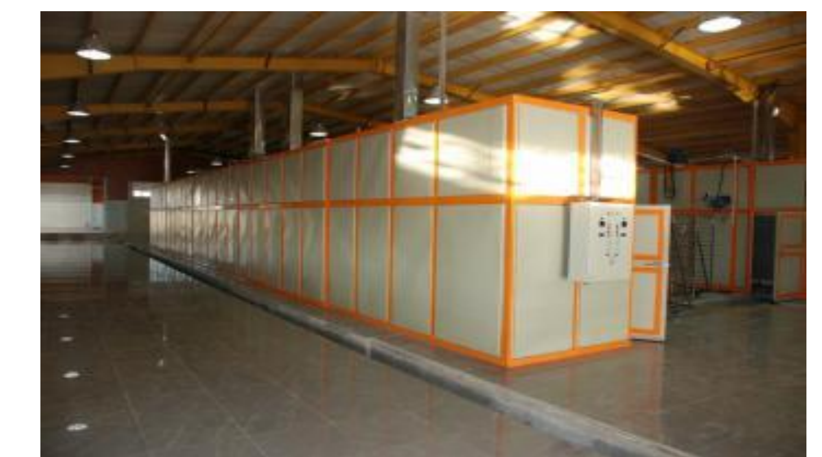
A continuous-throughput belt dryer in a saffron processing plant. Such dryers are very expensive but allow for high throughput and precise control.
