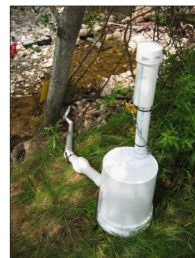
RAN researcher measures stream flow, and a stream gauge monitors water level of study streams.
