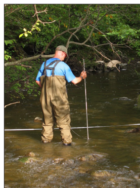
RAN researcher measures stream flow, and a stream gauge monitors water level of study streams.
