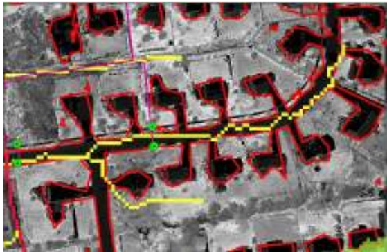
Figure 12. Impervious surfaces outlined based on the 2.44m multi-spectral Quick Bird image (red line) versus NDVI on the basis of 15cm MPO NIR image.
