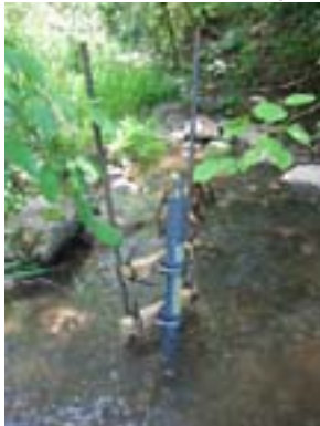
Munroe Brook YSI (attached to rebar in streambed)
