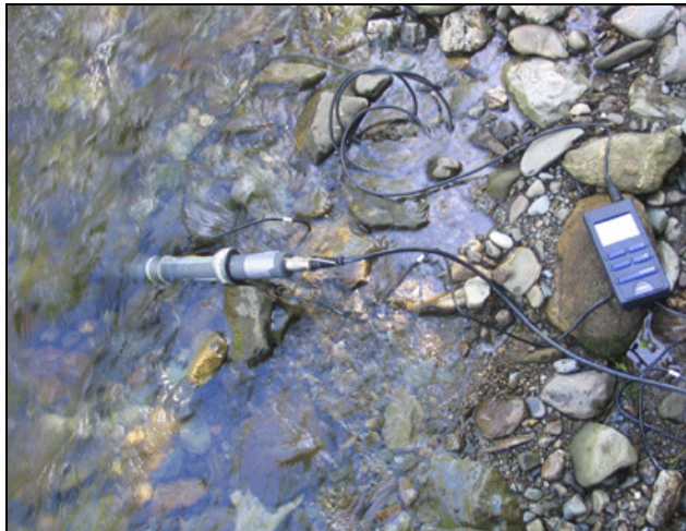
Figure 9. A DataSonde in position, used to collect physical and chemical stream water data ( www.uvm.edu/~ran ).
