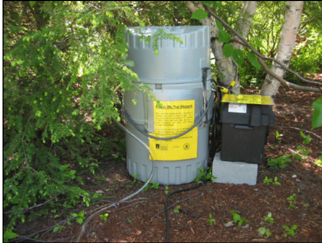
Figure 8. A picture of an ISCO automatic sampler in the field. Cables and tubing towards the bottom of the picture collect data and water samples from the stream which are then stored inside the sampling device ( www.uvm.edu/~ran ).
