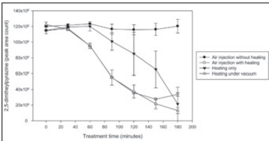
**Figure 2.** Mean ( $\pm$  standard error) quantity of 2,5-dimethylpyrazine (2,5-DMP) in maple syrup collected at 30-minute intervals during the application of four treatments investigated for efficacy in remediating metabolism off-flavor: air injection of syrup at ambient temperature, air injection of syrup during syrup heating, heating syrup in an open pan, and heating syrup while vacuum was applied.  $n=2$  at each timepoint.
