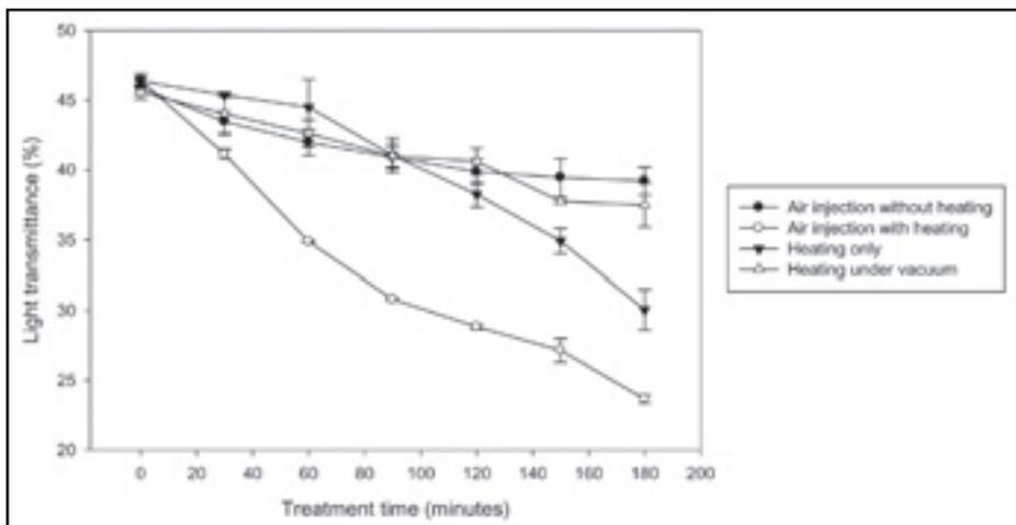
**Figure 3.** Mean ( $\pm$  standard error) percent light transmittance at 560nm of maple syrup collected at 30-minute intervals during the application of four treatments investigated for efficacy in remediating metabolism off-flavor: air injection of syrup at ambient temperature, air injection of syrup during syrup heating, heating syrup in an open pan, and heating syrup while vacuum was applied.  $n=2$  at each timepoint.
