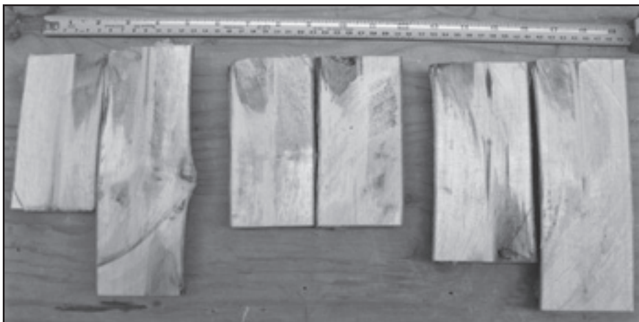
Figure 2. Internal staining in young maple stems tapped with regular (food-grade nylon) spouts and antimicrobial silver spouts. For each pair of stem segments, the regular spout is on the left and the antimicrobial silver spout is on the right. Note the very small stain pattern, probably the result of the slow growth and suppressed stature of these saplings.
