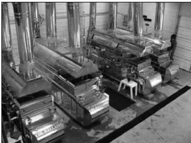
**Figure 1.** Research evaporators at the University of Vermont Proctor Maple Research Center Maple Processing Research Facility. Evaporators are oil-fueled, 3 x 10' with cross-flow pans and raised flues.
