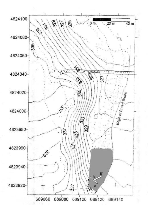
Figure DR4B. Topographic map of Bridgewater Corners fan. X and Y axes are in UTM coordinates. Contour interval is 1 meter. Dots are measured survey points. A-A' and B-B' are trench locations. Dashed line is stream channel.
