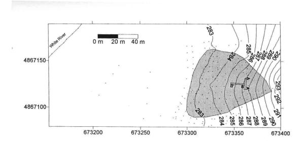
Figure DR3B. Topographic map of Hancock fan. X and Y axes are in UTM coordinates. Contour interval is 1meter. Dots are measured survey points. A-A' and B-B' are trench locations.
