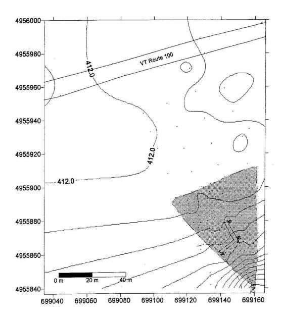
Figure DR1B. Topographic map of Eden Mills fan. X and Y axes are in UTM coordinates. Contour interval is 0.5 meter. Dots are measured survey points. A-A' and B-B' are trench locations. Dashed line is stream channel.
