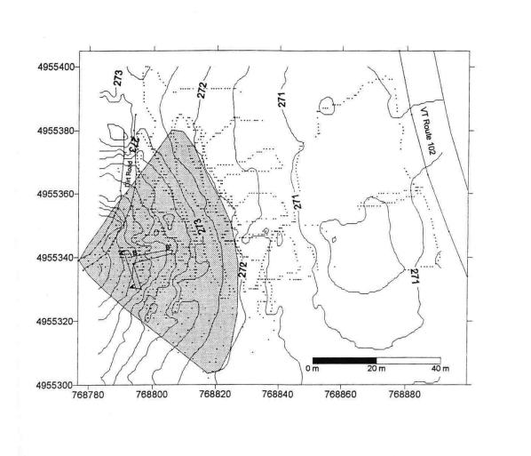
Figure DR5B. Topographic map of Maidstone fan. X and Y axes are in UTM coordinates. Contour interval is 1 meter. Dots are measured survey points. A-A' and B-B' are trench locations.
