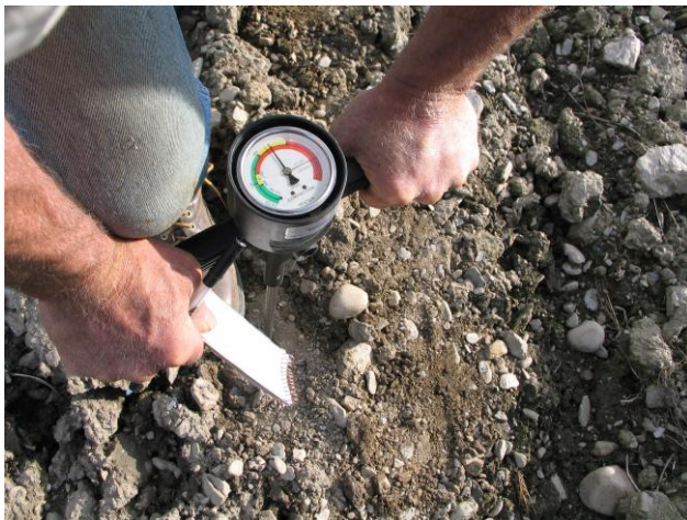
A penetrometer measures compaction in pounds per square inch of pressure. If it takes more than 300 psi to push through a compacted layer, it is unlikely that crop roots will be able to grow through the layer.
