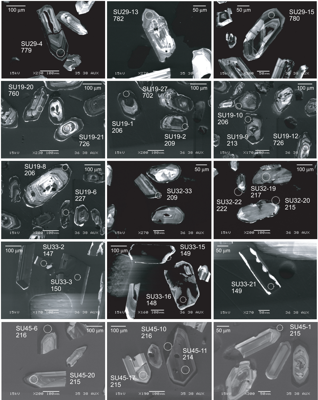
Figure 3. Cathodoluminescence (CL) images of representative analyzed zircons from each sample. Analysis number with corrected ^{206}\text{Pb}/^{238}\text{U} age and spot locations (dashed circles) correspond to those listed in Appendix 1. Streaking is due to charging on nonzircon grains.
