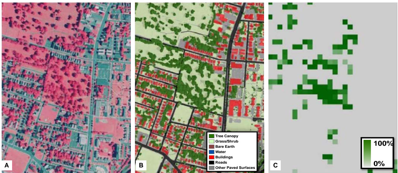
Figure 3. One-meter National Agricultural Imagery Program imagery (a) was used to derive high-resolution land cover data (b) for Hartford, CT. By capturing small, isolated patches of trees, this method estimated that 26% of the city's land area was occupied by tree canopy. In contrast, the 30-meter National Land Cover Dataset (c) estimated tree-canopy coverage of 15%.
