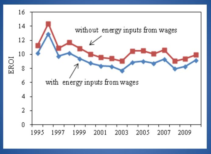
Sensitivity analysis for EROI<sub>stnd</sub> without and with energy inputs from wages
