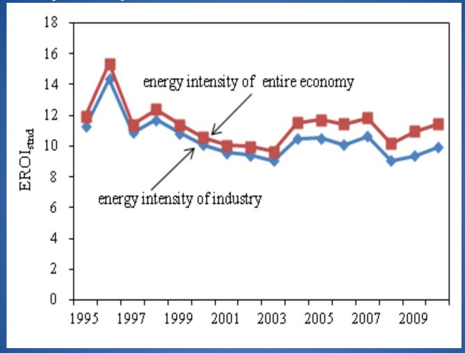
Sensitivity analysis for EROI<sub>stnd</sub> using the energy intensity for the entire economy and that of industry for estimating the indirect energy.
