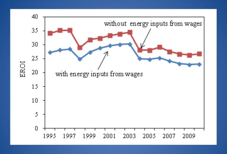
Sensitivity analysis for EROI<sub>stnd</sub> without and with energy inputs from wages
