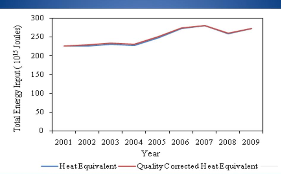
Results- Historical EROI of the Daqing oil field calculated in four different ways. The upper two lines do not include indirect energy costs.
