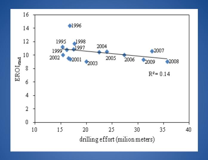
Relation of EROI<sub>stnd</sub> and drilling effort of oil and natural gas extraction in China with linear best fit
