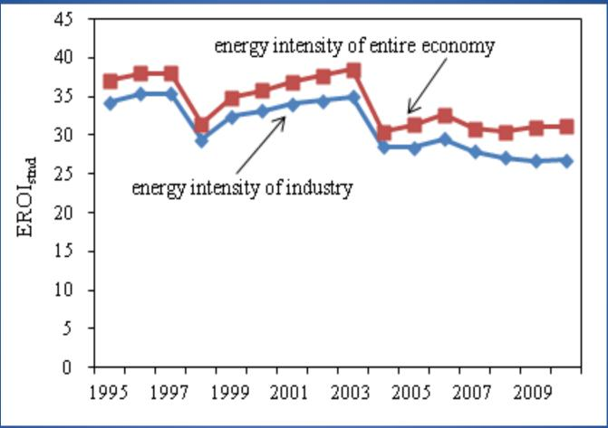
Sensitivity analysis for EROI<sub>stnd</sub> using the energy intensity of the entire economy and that of industry for estimating the indirect energy.
