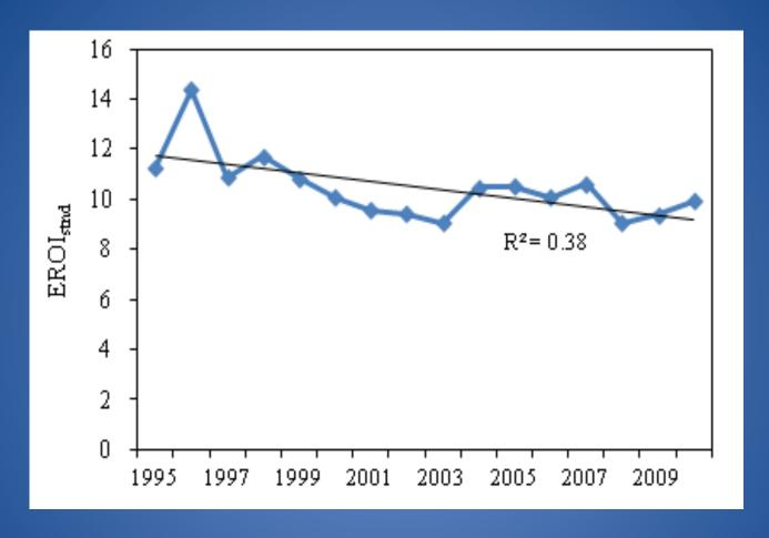
EROI<sub>stnd</sub> of oil and natural gas extraction in China with linear best fit
