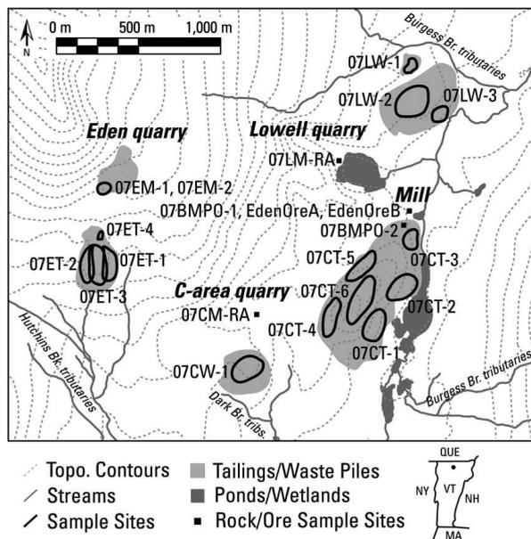
**FIGURE 1.** Site map showing tailings and waste piles, surface water features, and topography. Topographic contours are spaced at 30.5 m (100 ft). Sample collection sites are shown. The site is contained within two Lake Champlain watersheds. Hutchins Brook flows into Dark Branch, which is in the Lamoille River watershed, and Burgess Branch is in the Missisquoi River watershed.
