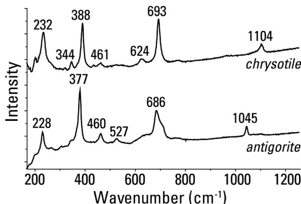
**FIGURE 3.** Raman spectra of two mineral grains from sample 07EM-2. Peaks are labeled by wavenumbers. These spectra were used to establish the presence of two minerals with similar composition and XRD peaks. Data were compared with published patterns (Rinaudo et al. 2003), RRUFF database patterns (Downs 2006), and those of reference samples.
