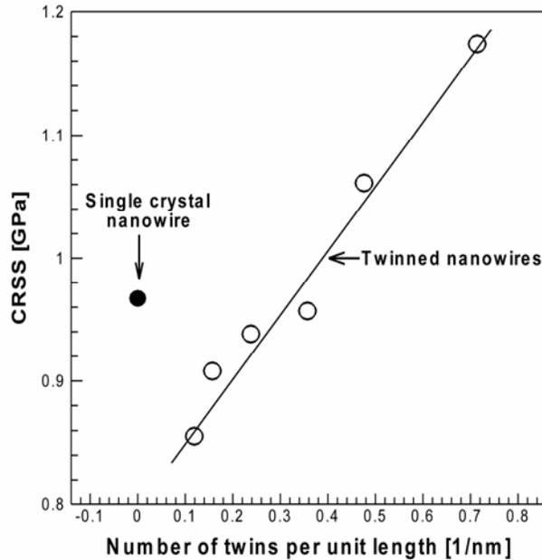
**Fig. 3.** Linear dependence of the critical resolved shear stress (CRSS) at yield point on the number of preexisting twins per unit length in Au nanowires with a diameter of 12.3 nm. The CRSS value for a single-crystal nanowire with corresponding diameter is shown for comparison.
