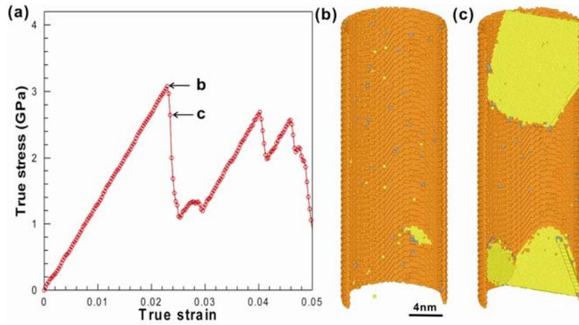
**Fig. 1.** Tensile behavior of a single-crystal, defect-free Au nanowire with a diameter of 12.3 nm from molecular dynamics simulation. (a) Simulated stress-strain curve. (b) Surface dislocation emission at yield point. (c) Propagation of  $1/6\{11\bar{1}\}\langle 112\rangle$  partial dislocations followed by strong strain softening effects in the post-yielding stage. (b)-(c) Only non-FCC atoms and one half of the nanowire model are represented for clarity.
