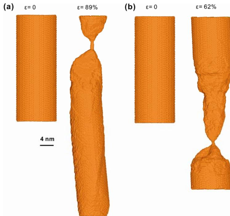
**Fig. 4.** Simulated fracture of Au nanowires of 12.3 nm in diameter. (a) Single-crystal, defect-free nanowire. (b) Twinned nanowire with 4.2 nm-twin boundary spacing. The loading direction is vertical for all nanowires.
