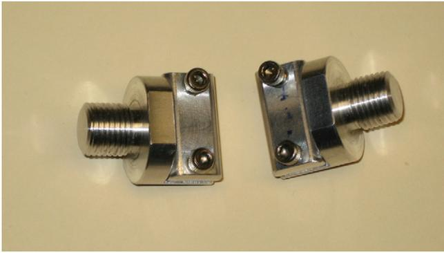
Fig. 3. Holder used for high strain-rate tests.
