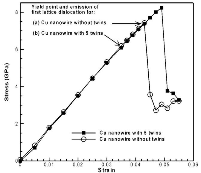
FIG. 1. Tensile stress-strain curves for single crystal and five-twin Cu nanowires as obtained from the same computational procedure used by Cao *et al.* The yield point corresponding to the emission of the very first lattice dislocation is indicated by an arrow.
