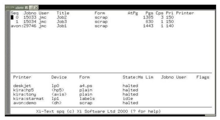
To operate upon a job or printer, it should be selected by moving the cursor to it and typing one of various single-keystroke commands.
