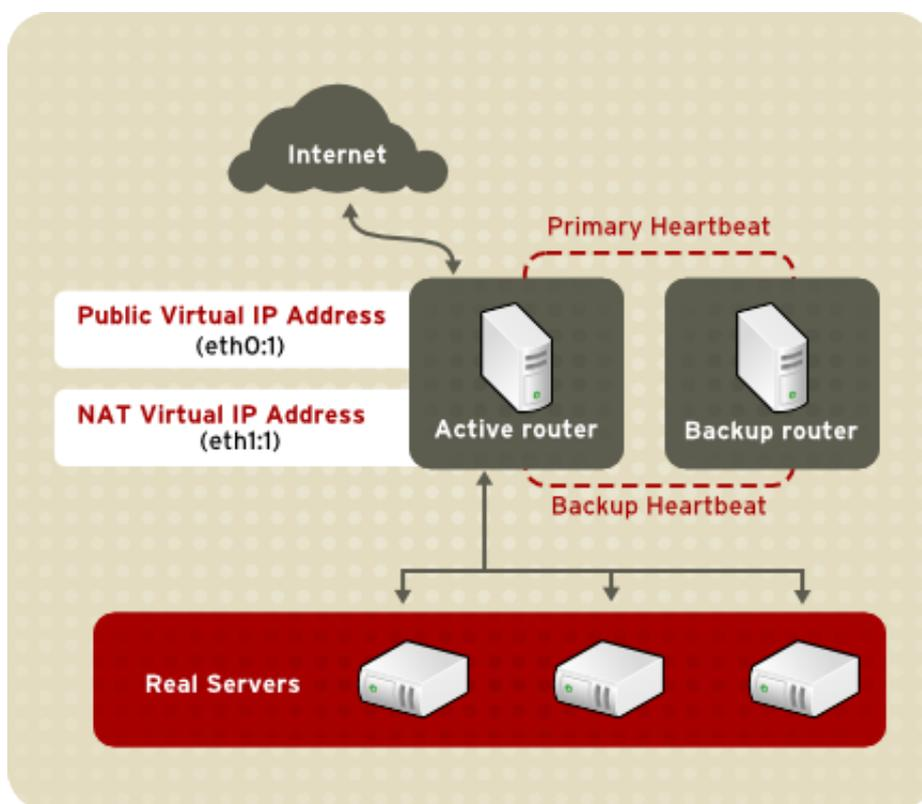
Figure 1.3. Load Balancer Add-On Implemented with NAT Routing
