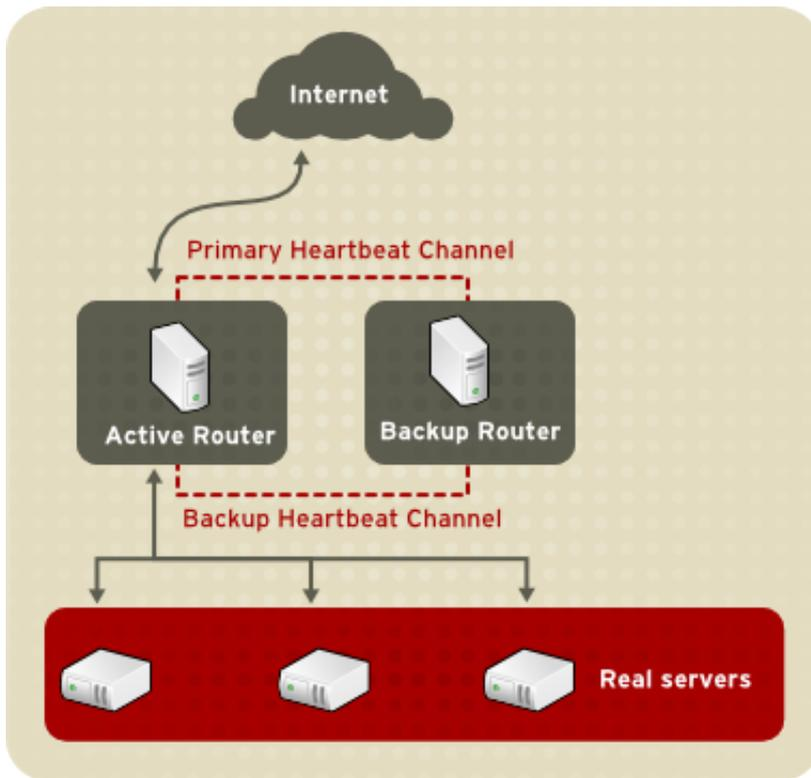
Figure 1.1. A Basic Load Balancer Add-On Configuration
