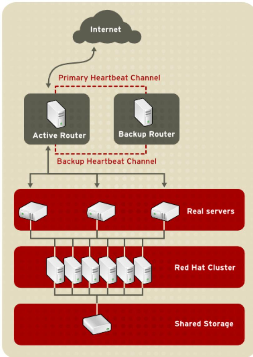
Figure 1.2. A Three-Tier Load Balancer Add-On Configuration
