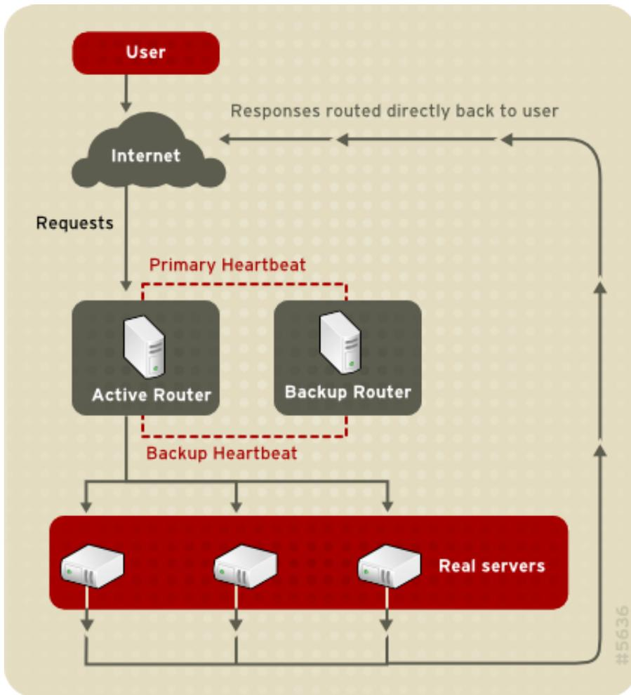
Figure 1.4. Load Balancer Add-On Implemented with Direct Routing
