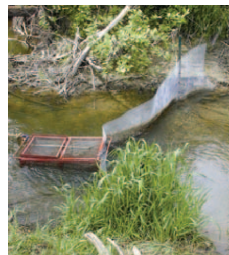
A portable assessment trap captures sea lamprey as they swim upstream to spawn.
