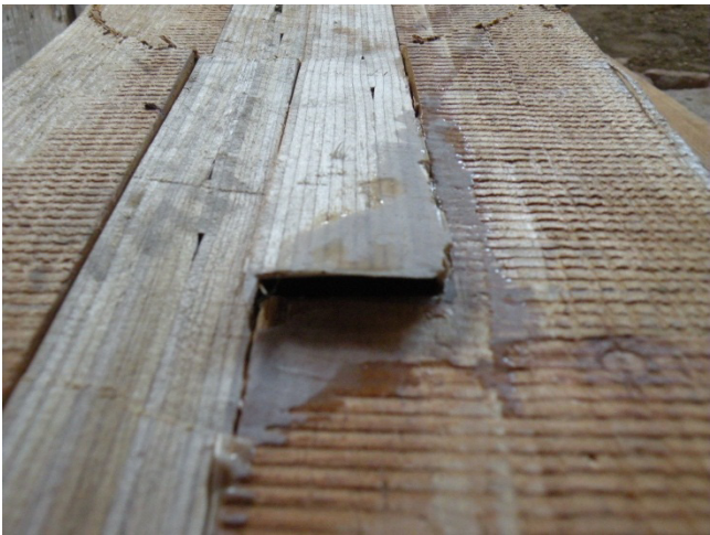
Figure 5. Poor-quality LVL Dutchman repair specimen after failure.
