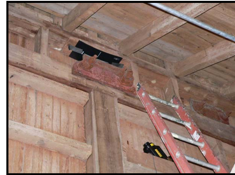
Figure A. Setup for digital radioscopy examination of a post-beam connection.
