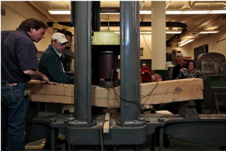
Figure 12 – Full size samples were tested to compare the performance of repaired timber to undeteriorated timber.
