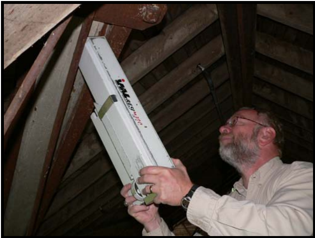
Figure 3. Use of the IML-RESI System to inspect a timber.
