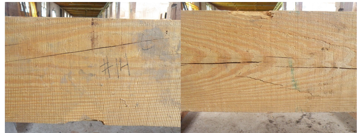
Figure 2. Control sample with moderate slope of grain (on the left) and failure on the tension zone (on the right).
