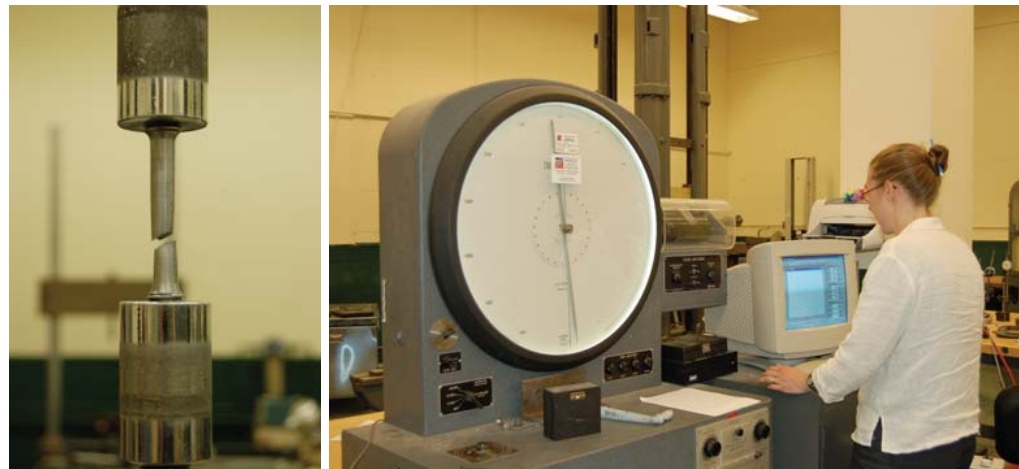
Figure 5: Tension tests (ASTM A 370-97a) were conducted on iron samples, yielding average peak stress values of approximately 319,820.7 KPa.
