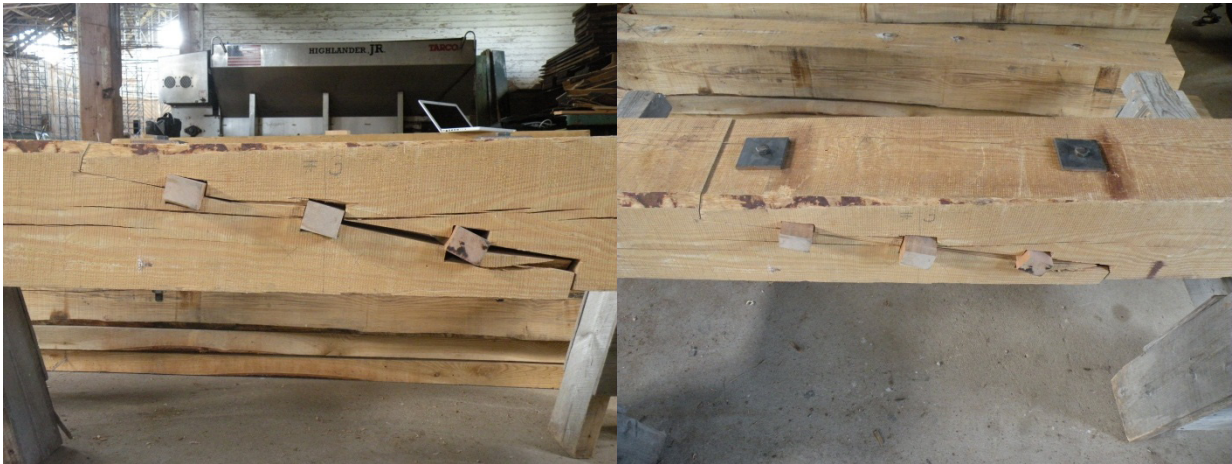
Figure 3. Failure of a scarf joint repair specimen.
