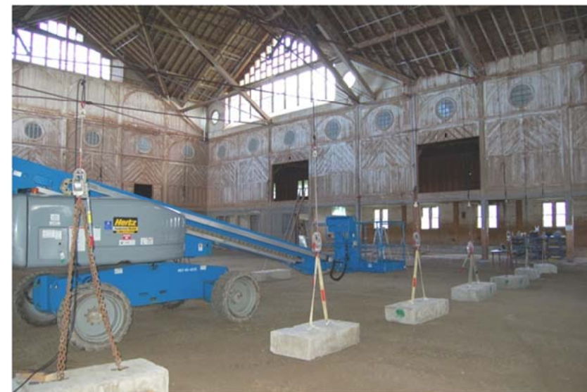
Figure 8 – Two trusses were load tested. Loads were applied at purlins, and changes in strain were recorded. Results were compared to computer models of the truss.
