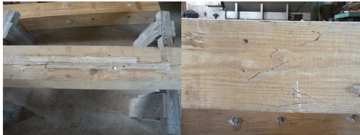
Figure 4. High-quality LVL Dutchman repair specimen after failure.
