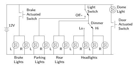
The designer of such a network needs to answer questions such as: how much electricity flows when both the hi-beam headlights and the brake lights are on? We will use linear systems to analyze simple electrical networks.
