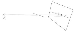
This is a *central projection* from a single point. As the sketch shows, this projection is not orthogonal like the ones we have seen earlier because the line from the viewer to C is not orthogonal to the image plane. (This model is only an approximation—it does not take into account such factors as that we have binocular vision or that our brain's processing greatly affects what we perceive. Nonetheless the model is interesting, both artistically and mathematically.)
