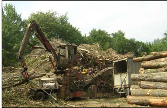
Tree tops and limbs are severed from the log portion and sorted into piles at the landing
