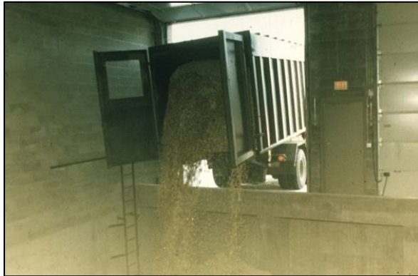
Chips are unloaded from trailers into chip storage bins
