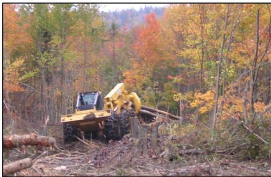
Grapple skidders are used to drag felled trees to a central staging area or "landing"
