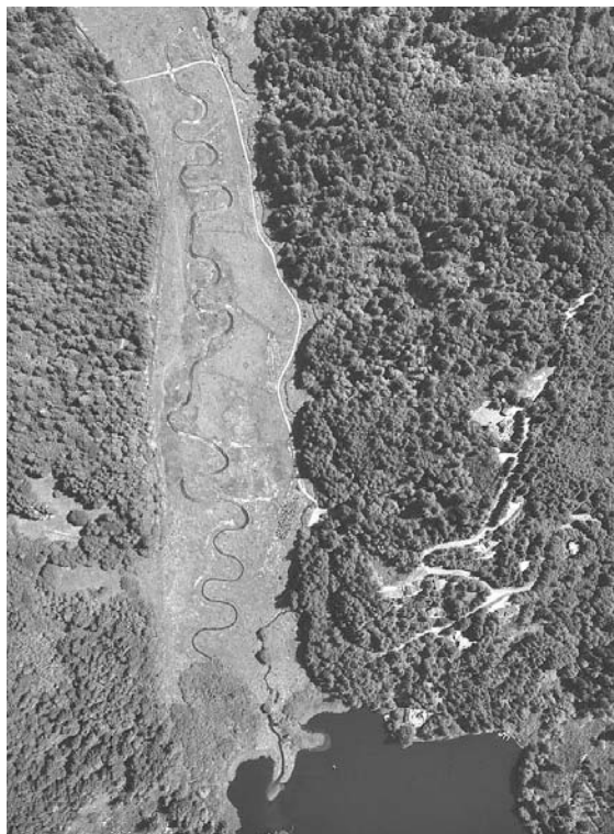
Figure 1. Low-elevation aerial photograph of the new Bailey Creek channel before connection to the old ditch, September 2000.
