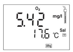
2 Switch the salt content correction off with <▼>. The SAL display indicator is no longer displayed.
