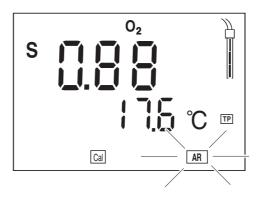
As soon as a stable value is reached, the *AR* display indicator stops flashing. This indicates that the calibration is complete; the sensor symbol shows the relative slope that was determined and the sensor evaluation (see page 20).
